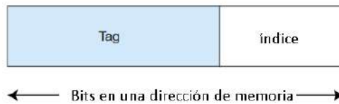
FIGURE 6.8 The Main Memory Address Format for Associative Mapping
