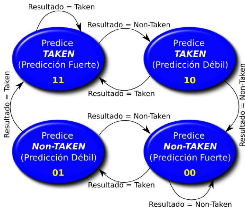
Figura 2.9: Branch Prediction Buffer - 2 bits
