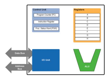
The following diagram, along with some of the current discussion, was adapted from my first P4 vs. G4e article. It shows three different execution units: the load-store unit (LSU), the integer or arithmetic-logic unit (ALU), and the floating-point unit (FPU). Since we haven't yet talked about putting more than one execution unit in the processor, just ignore the LSU and FPU for now. They'll show up again in the next section.
